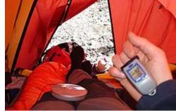
ng an oximeter. This instrument can be a useful indicator of altitude problems
